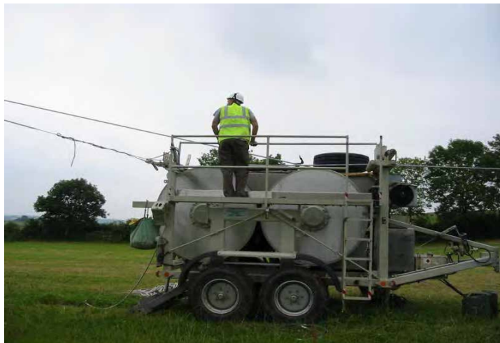
Figure 5.7 Puller – Tensioner Machine
